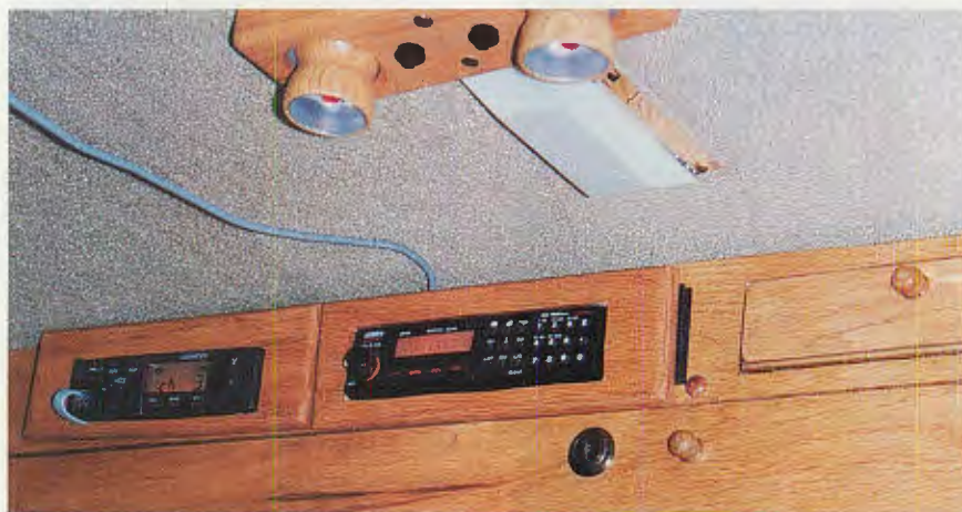
Modern-day, mission-specific features of Anderson's customized operations van include this overhead console: two-way radio at left, police scanner at center over weapons locker. Ceiling holds battle-lantern assembly for night operations.
